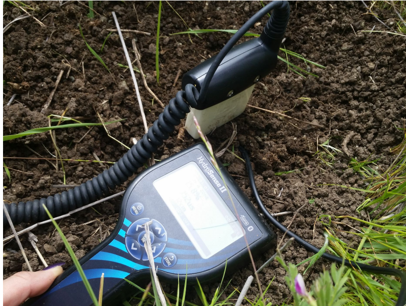
Comparing our soil moisture sensor with a HydroSense II soil-water sensor
